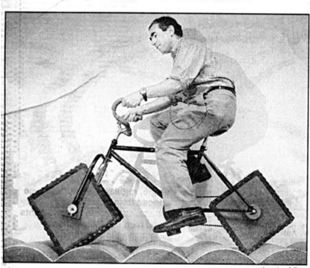
Math professor Stan Wagon demonstrates his square-wheeled bicycle at Macalester College in St. Paul, Minn. In 1966, it was discovered that a square wheel would roll smoothly on a road made of catenaries (those humpy things). Wagon said he became interested in the concept 7 years ago, did calculations and computer animations, then had the bike specially built.
