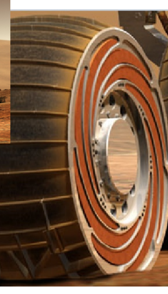
Spiral springs wheel used by NASA on its rovers Spirit and Opportunity in 2004
