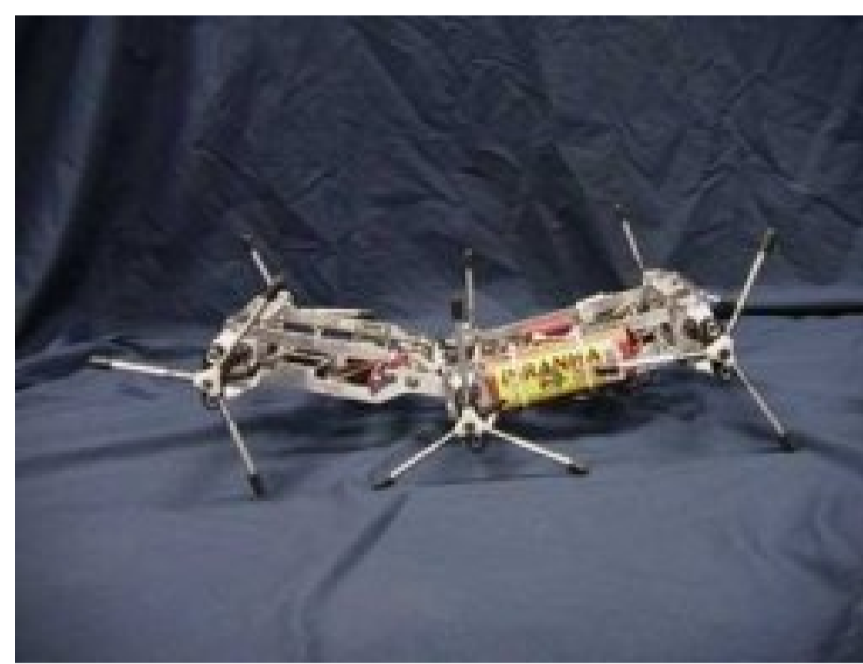
Whigs (Wheels and legs) Biorobots: 1 st & 2 nd generations inspired by the cockroach locomotion Case Western Reserve University, Ohio
